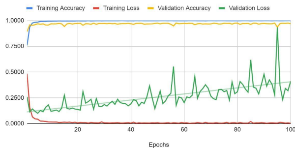
Figure 6: Training and Validation Metrics for L2 Regularization + Two 0.5 Dropout Layers
