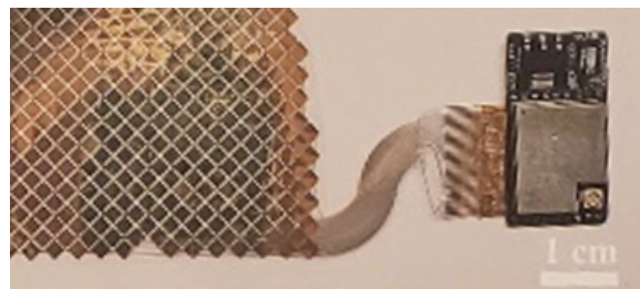
Figure 3. unpacked sensor array and PCBs
