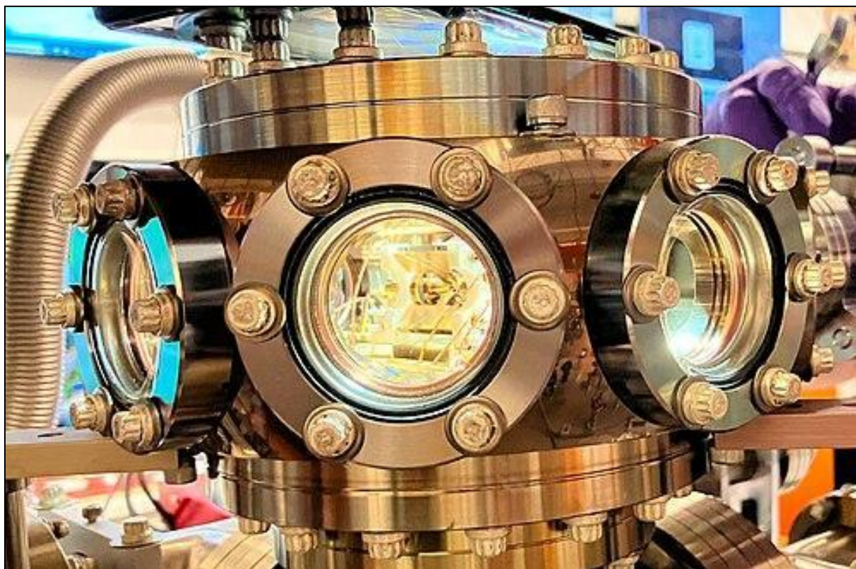
Figure 3: A Paul ion trap, used for precision measurements of radium ions, inside a vacuum chamber.
